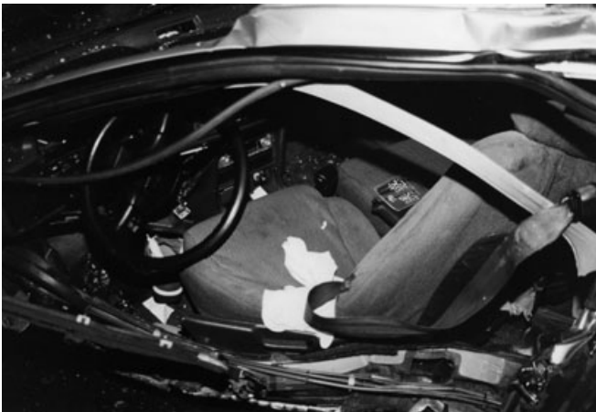
FIG. 1—1990 Acura Integra showing drivers side after the collision. The 2-point restraint is intact. The lap belt is not engaged.
